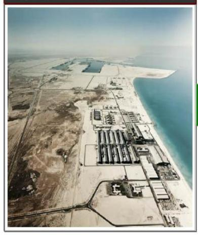
Sevenfold capacity increase in 30 years The DUBAL Smelter Complex in 2010: 8 potlines with a combined capacity of 1 million mtpa
